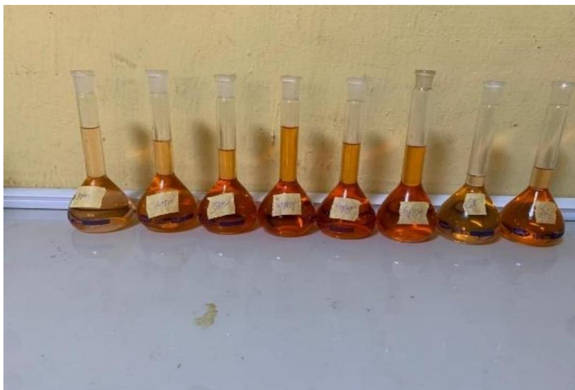
Figure 8: Standard (a-f) and sample solutions (g-h) after complexing with 1,10-phenanthroline
